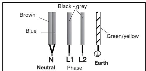
With hook-up of 400 V 2N three phase, verify that the neutral wire is properly connected
