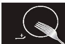
**"Small Items" safety.** By placing a small object on the area (a ring, a fork, etc), the hob will detect it and not deliver any power. The power display flashes. Note: However, several small objects at the same time on a zone could be identified as cookware. In that case, power will be delivered by the hob. Do not place any utensils (spoons, forks, covers, etc) on the cooking zone being used. They will heat up in the same way as cookware: Risk of combustion.
