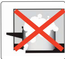
**Protection against overflows.** In case of overflow, or of a metallic object or wet cloth placed on the control areas, the hob turns itself off, the displays light up and a beep sounds. Clean the hob or remove the object, then begin cooking again.
