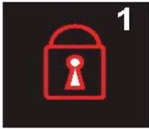
**Child Lock:** for added peace of mind, the child lock can be manually activated to prevent accidental start-up. To activate the lock pres the “I” key and hold until a beep is sounded and an indicator appears. To de-activate hold the “I” key until the indicator goes out and a beep sounds.
