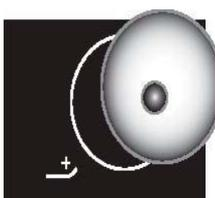
**Automatic Pan Detection:** detects when a suitable pan is placed on the cooking zone and so eliminates the possibility of the hob being activated accidentally by a non-suitable object.
