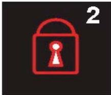
**Control Lock:** can be activated to lock the control panel during the cooking process. This will lock the controls set on the cooking zones but will allow the stop key to function. This is activated in / deactivated in the same way as the child lock.
