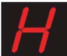
**Residual heat.** After a long cooking period, the zone used can remain hot for several minutes. An "H" flashes during this period. Do not put your hand on the zone.
